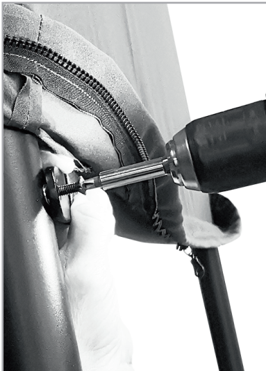
4. Screw the flat bars to the frame.
