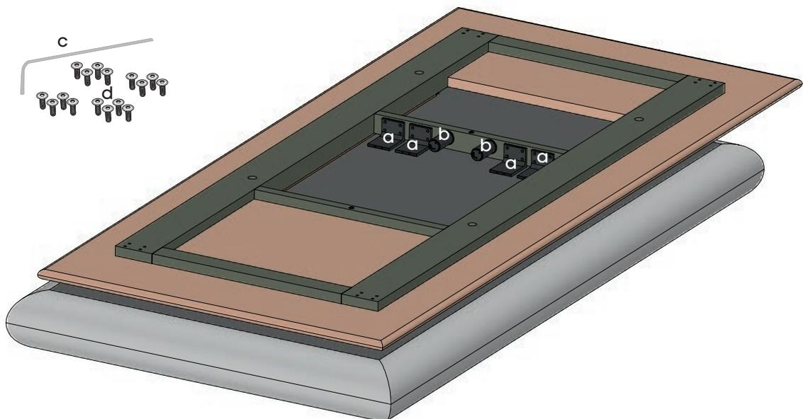
3. Position each of the 4 Feet (a) on the 4 bores (e) and tighten them with 4 screws.
