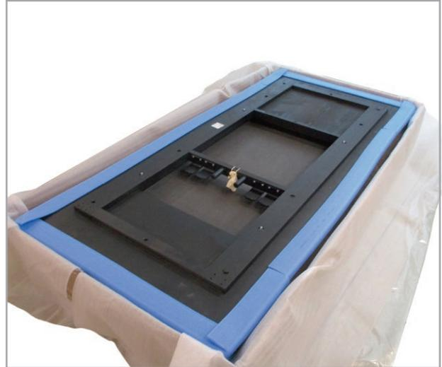
2. Unscrew the 4 feet (a) from the plateau using the Allen key (c) supplied and unscrew also the 2 support feet (b). Lay out the feet and screws (d) removed from the plateau and the screws (d) supplied in front of you.
