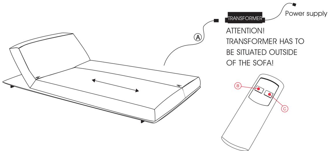
To avoid traces of usage at cover material, seat should (as possible) only be adjusted when back and armrest are folded up (like fig. above).
