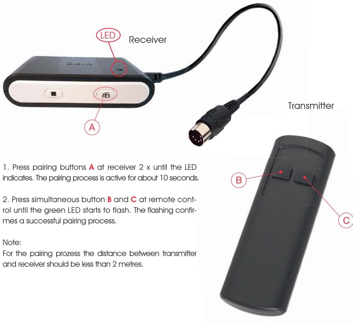
1. Press pairing buttons **A** at receiver 2 x until the LED indicates. The pairing process is active for about 10 seconds.
