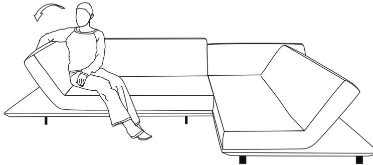
2. To obtain zero position pull the armrest carefully beyond the top position into your direction and fold down into zero position.
